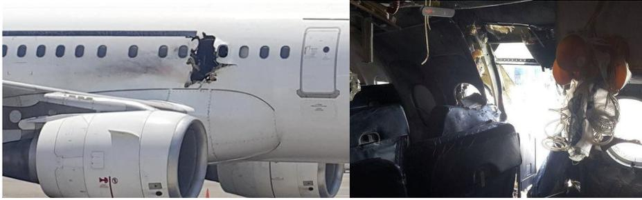
Interior and Exterior Views of Laptop Bomb Damage to Daallo Airlines Flight 159
